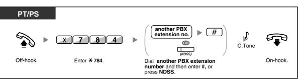
• To restart monitoring of an extension after performing this operation, go off-hook, press the corresponding NDSS button, and go on-hook.
