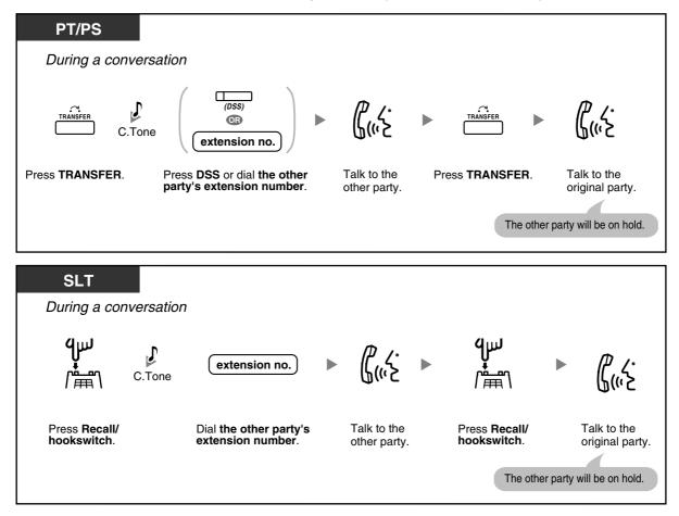
PT/PS During a conversation ۲. ۲.) (DSS) J TRANSFER OR C.Tone extension no. Press DSS or dial the other Press TRANSFER. Talk to the Press TRANSFER. On-hook. party's extension number. other party. SLT During a conversation ٩w ٩w J ¶ر:∠ ل\_ښځ extension no. C.Tone Г Ħ Press Recall/ hookswitch. Dial the other party's extension number. Press **Recall/** hookswitch. On-hook. Talk to the other party.
