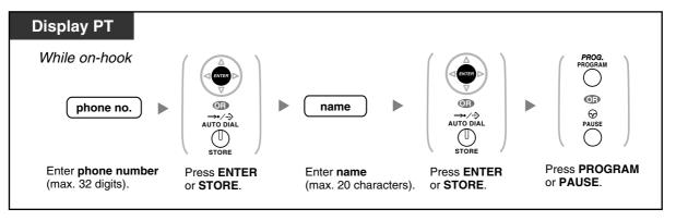
• Telephone numbers and names displayed are stored using the first spare Personal Speed Dialling memory available.
