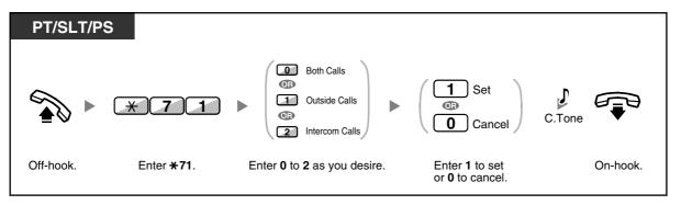
When using a proprietary telephone, you can set or cancel Do Not Disturb by pressing the FWD/DND button (fixed button) instead of "×710".
